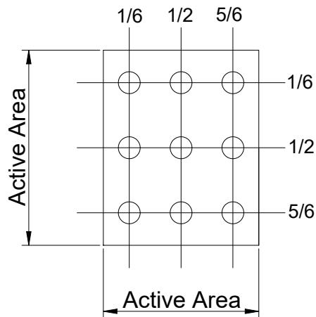
$$U_n = \frac{B_{min}}{B_{max}} \times 100\%$$
