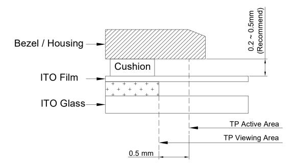
The corner part has conductivity. Do not touch any metal part after mounting.
